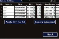
Set unused camera FPS speeds to Off, so the DVR will not generate video loss events.
