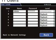
Users logging on to the DVR locally or remotely should have password control to protect the DVR from being accidentally reconfigured.
