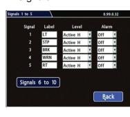
Label: For signals 1-5, select from: LT left turn, STP stop, BRK brake, WRN warning light, and RT right turn.
