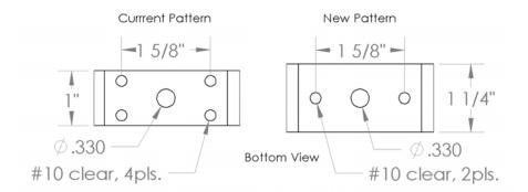
**Reason for Change:** A wider mounting surface area for better stability, and a reduced number of mounting holes ensures quicker and easier installation.
