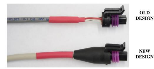
**Reason for Change:** This change was implemented to better protect and act as a water seal. This redesign also helps to maintain the wiring integrity by preventing overly straining the wiring from tension, or pulling between the wiring and the connector.
