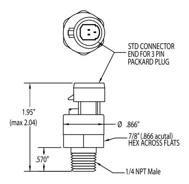
This drawing is valid for pressure sensors with the following FRC part numbers: XE-WLPT3-Sxx, XE-WLPT30-Sxx,
