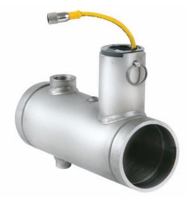
The FoamPro foam manifold incorporates the flowmeter sensor, main waterway check valve, concentrate injection port and drain port all into one compact assembly. Each manifold is tested to 500 psi to guarantee integrity and is delivered with FoamPro's unmatched accuracy.
