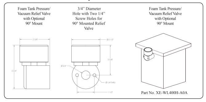
**NOTE**: *Relief valve must be mounted in a vertical position*. The valve can not be immersed in foam. (If there is no fill tower, mount the valve at the highest point of the tank top so that it is not immersed in foam.)
